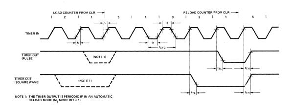
Figure 15. Timer Output Waveform Countdown from 5 to 1
